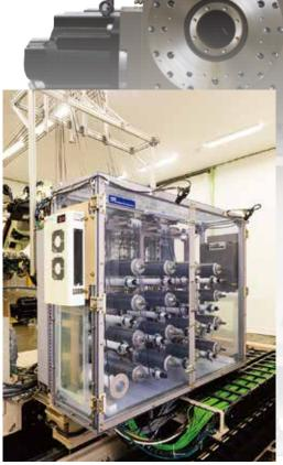
TFL uses thermoset prepreg slit tape. 16 spools can be installed in the creel box as standard. Those tapes are delivered to the head at optimized tension control. TSUDAKOMA's tension control technology was originally developed for textile machines. High quality slit tapes can be produced using our TPS prepreg slitter.
